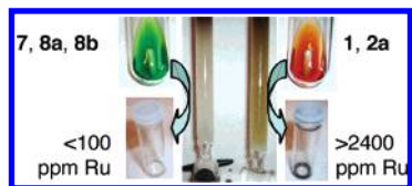
Figure 1. Purification of RCM product 10 (5 mol % Ru) by silica gel chromatography. 5% EtOAc:hexanes: 7 , 8 : <100 ppm Ru ( 1 : 30 900; 2a : 57 900 ppm). 15% EtOAc:hexanes: 1 : 2450 ppm Ru ( 7 : 600 ppm).
