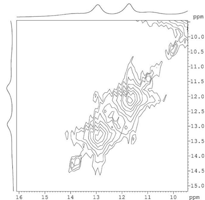
Fig. 2. Magnitude  ${}^1H$  COSY spectrum of complex **5** at 200 MHz at 20 °C in  $d_6$ -acetone solution recorded with a delay time of 150 ms. Only the region relevant to the assignment of pyridyl resonances is shown in the top trace.
