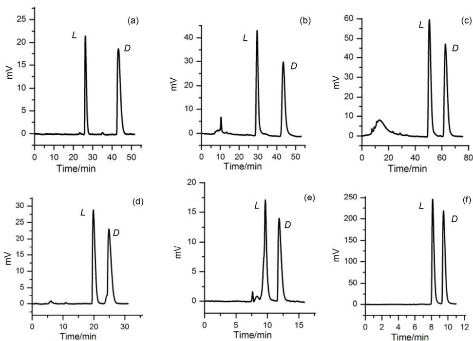
**Figure 3** Representative chromatograms of  $\alpha$ -amino acids on the CSP-1 (250 mm long  $\times$  4.6 mm i.d.): (a) phenylglycine, (b) 4-hydroxyphenylglycine, (c) tyrosine, (d) methionine, (e) glutamic acid, and (f) histidine using a perchloric acid solution (10 mmol/L, pH = 2) as the mobile phase at a flow rate of 0.5 mL  $\cdot$  min $^{-1}$  at 25 °C. The signals were monitored with a UV detector at 210 nm.
