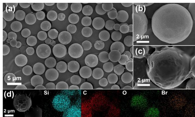
**Figure 2** (a) SEM image of silica spheres; (b) SEM image of the  $C_{18}$  silica before coating its surface; (c) SEM image of the coated surface; (d) a close view of the detailed features of the **CSP-1** electrode, along with the (Si, C, O, Br) corresponding EDS element mapping of the silica composite.
