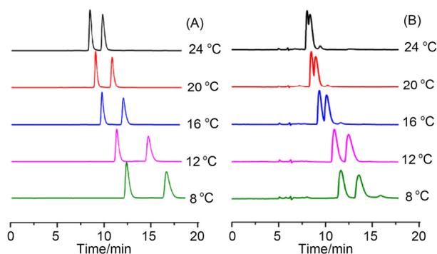
**Figure 4** Chromatograms on the **CSP-1** packed column for the separation of (A) histidine and (B) serine at 8–24 °C. Perchloric acid solution (10 mmol/L, pH=2) as the mobile phase, flow rate of 0.5 mL·min<sup>-1</sup> and with UV detection at 210 nm.
