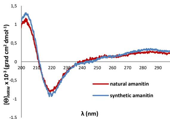
Figure 2. CD spectra of natural and synthetic  $\alpha$ -amanitin (1).
