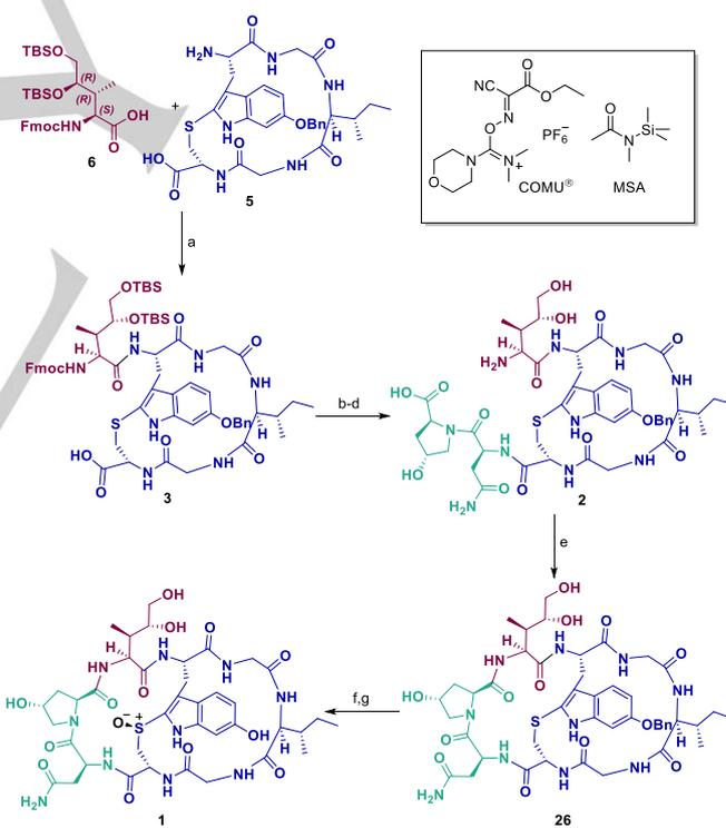
**Scheme 5.** Fragment couplings and cyclizations to the target molecule  $\alpha$ -Amanitin (**1**): a) MSA, COMU, DIPEA, DMA, 0°C to r.t. 3 h; b) (a and b: one pot), H-Asn-Hyp-OFm·HCl (**4**), HATU, DIPEA, DMF, 0°C to r.t., 2 h; c) Et<sub>2</sub>NH, DMF, 1 h, r.t.; d) 1 M TBAF, THF, r.t., 2 h, 77% over four steps; e) HATU, DIPEA, DMF, r.t., 16 h, 68%; f) BF<sub>3</sub>·OEt<sub>2</sub>, EtSH, r.t., 2 h; g) *m*CPBA, *i*PrOH/EtOH (2:1), r.t., 30 min, 35% over two steps.
