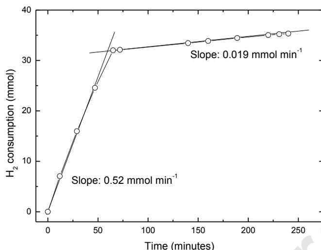
Fig. 4. Hydrogen consumption profile of nitrobenzene hydrogenation. Run conditions: reaction volume 20 mL, nitrobenzene 0.5 mol L<sup>-1</sup>, Hydrogen Pressure 0.8 MPa, NH<sub>2</sub>OH·HCl 30 mmol, T 333 K, Pd/C 50 mg.
