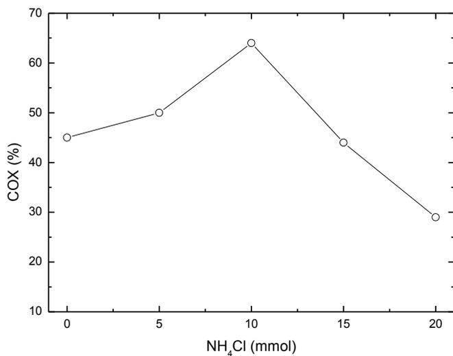
Fig. 10. Influence of  $\text{NH}_4\text{Cl}$  amount on COX yield. Run conditions: reaction volume 20 mL, AN 0.5 mol L<sup>-1</sup>, Hydrogen Pressure 0.8 MPa,  $\text{NH}_2\text{OH}\cdot\text{HCl}$  30 mmol,  $\text{H}_2\text{O}$  20 mmol, T 333K, Pd/C 50 mg, time of reaction 20 h.
