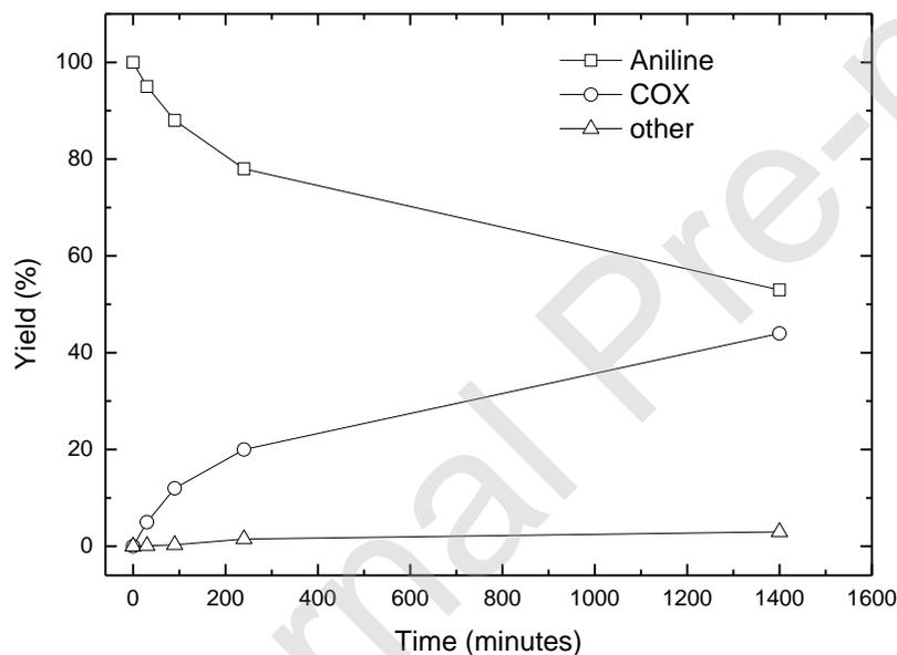
Fig. 6. Reaction profile of aniline hydrogenation. Run conditions: reaction volume 80 mL, aniline  $0.5 \text{ mol L}^{-1}$ ,  $\text{H}_2\text{O}$  20 mmol, hydrogen Pressure 0.8 MPa,  $\text{NH}_2\text{OH}\cdot\text{HCl}$  75 mmol, T 333K, Pd/C 50 mg.
