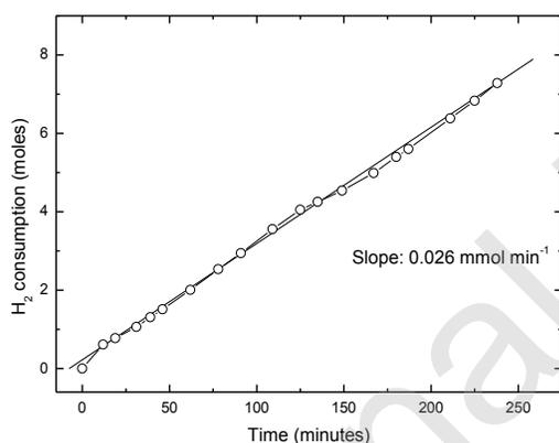
Fig. 5.  $\text{H}_2$  consumption profile for  $\text{NH}_2\text{OH}$  hydrogenation. Run conditions: reaction volume 20 mL, Hydrogen Pressure 0.8 MPa,  $\text{NH}_2\text{OH}\cdot\text{HCl}$  30 mmol,  $\text{H}_2\text{O}$  20 mmol, T 333K, Pd/C 50 mg.
