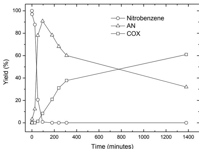
Fig. 2. Hydrogenation profile. Run conditions: reaction volume 75 mL, nitrobenzene 0.5 mol L<sup>-1</sup>, Hydrogen Pressure 0.8 MPa, NH<sub>2</sub>OH·HCl 75 mmol, T 333K, Pd/C 60 mg, time of reaction 20 h.
