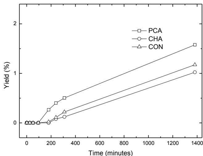
Fig. 3. Yields of low concentration products. Run conditions: reaction volume 75 mL, nitrobenzene 0.5 mol L<sup>-1</sup>, Hydrogen Pressure 0.8 MPa, NH<sub>2</sub>OH·HCl 75 mmol, T 333K, Pd/C 50 mg, time of reaction 20 h.
