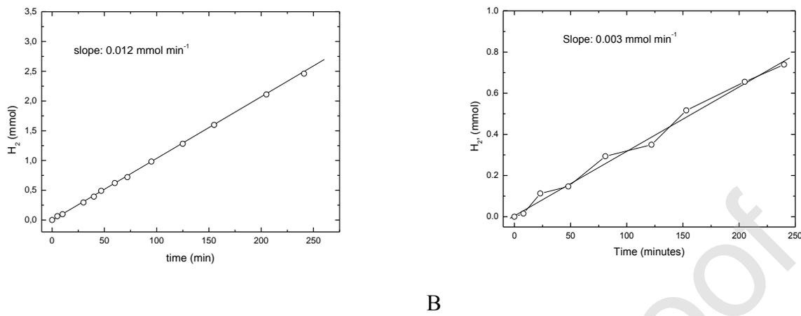
Fig. 7. Reaction profile of hydrogen consumption for AN hydrogenation. Run conditions: reaction volume 20 mL, aniline 0.5 mol L<sup>-1</sup>, H<sub>2</sub>O 20 mmol, hydrogen Pressure 0.8 MPa, T 333K, Pd/C 50 mg. A), reaction in the presence of 30 mmol of NH<sub>2</sub>OH·HCl; B) no NH<sub>2</sub>OH·HCl.
