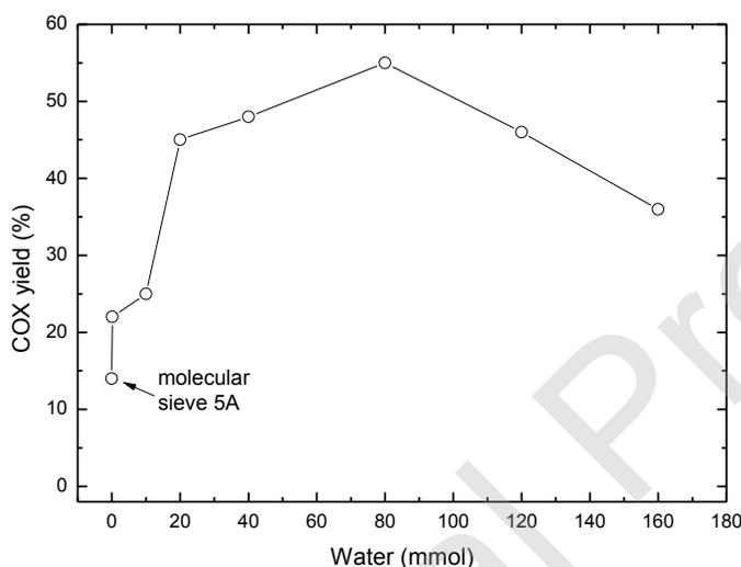
Fig. 9. Influence of  $\text{H}_2\text{O}$  on COX yield. Run conditions: reaction volume 20 mL, AN  $0.5 \text{ mol L}^{-1}$ , Hydrogen Pressure 0.8 MPa,  $\text{NH}_2\text{OH}\cdot\text{HCl}$  30 mmol, T 333K, Pd/C 50 mg, time of reaction 20 h.
