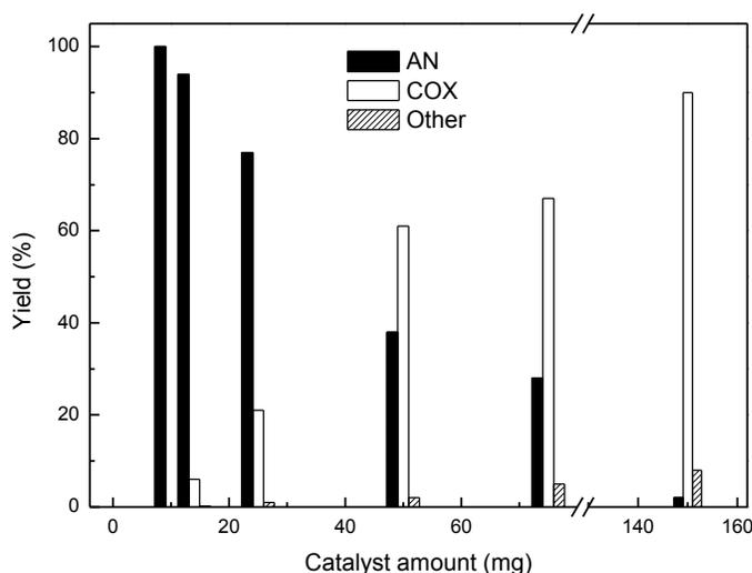
Fig. 1. Influence of the catalyst amount on the yield of aniline and cyclohexanone oxime. Run conditions: reaction volume 20 mL, nitrobenzene  $0.5 \text{ mol L}^{-1}$ , Hydrogen Pressure 0.8 MPa,  $\text{NH}_2\text{OH}\cdot\text{HCl}$  30 mmol, T 333K, Pd/C 50 mg, time of reaction 20 h.
