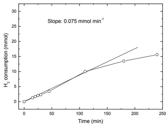
Fig. 8.  $\text{H}_2$  consumption profile for  $\text{NH}_2\text{OH}$  hydrogenation in the presence of  $0.5 \text{ mol L}^{-1}$  CHA. Run conditions: reaction volume 20 mL, Hydrogen Pressure 0.8 MPa,  $\text{NH}_2\text{OH}\cdot\text{HCl}$  30 mmol,  $\text{H}_2\text{O}$  20 mmol, T 333K, Pd/C 50 mg, time of reaction 4 h.
