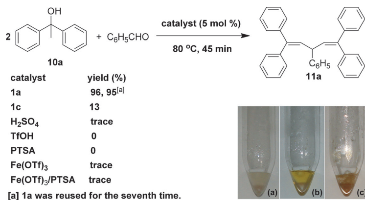
Figure 5. Reaction of benzaldehyde with 10a (Photos are taken at 80 °C, (a) 5 min; (b) 15 min; (c) at the end of the reaction).
