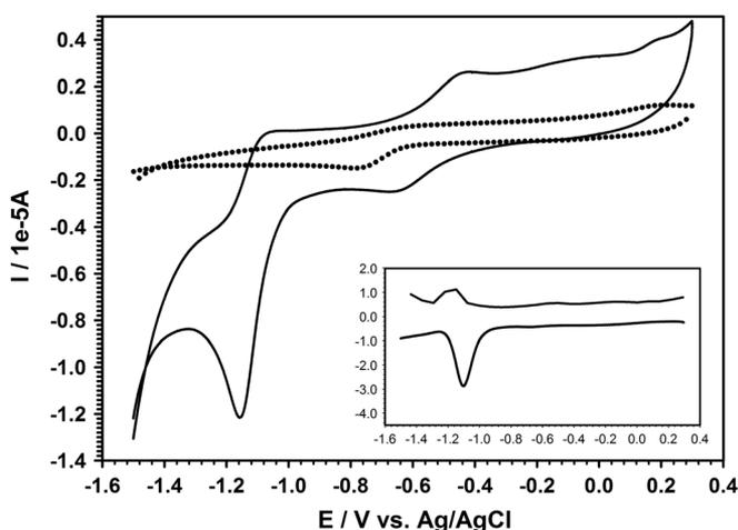
**Figure 2.** Cyclic voltammograms of Schiff base ligand **2** (dotted curve) and Pd(II) complex **2a** (solid curve) in DMF–LiClO<sub>4</sub> using glassy carbon electrode with  $0.1 \text{ V s}^{-1}$  scan rate (inset: square wave voltammogram of **2a**: amplitude, 50 mV; frequency, 15 Hz; glassy carbon working electrode).
