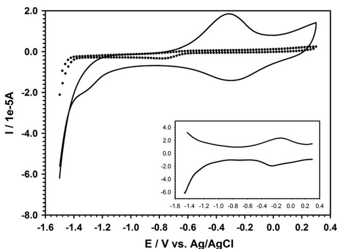
**Figure 3.** Cyclic voltammograms of Schiff base ligand **3** (dotted curve) and Pd(II) complex **3a** (solid curve) in DMF–LiClO<sub>4</sub> using glassy carbon electrode with  $0.1 \text{ V s}^{-1}$  scan rate (inset: square wave voltammogram of **3a**: amplitude, 50 mV; frequency, 15 Hz; glassy carbon working electrode).
