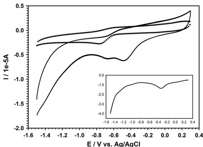
**Figure 1.** Cyclic voltammograms of Schiff base ligand **1** (dotted curve) and Pd(II) complex **1a** (solid curve) in DMF–LiClO<sub>4</sub> using glassy carbon electrode with 0.1 V s<sup>-1</sup> scan rate (inset: square wave voltammogram of **1a**: amplitude, 50 mV; frequency, 15 Hz; glassy carbon working electrode).
