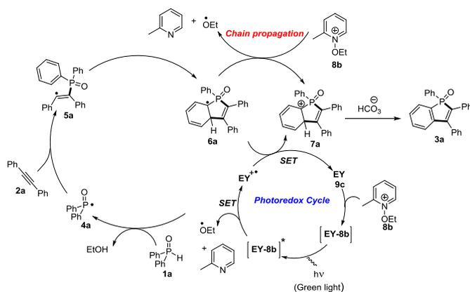
**Figure 7.** Postulated mechanism for the synthesis of the benzo[*b*]phosphole oxides **3a** via photoredox catalysis. EY: eosin Y.
