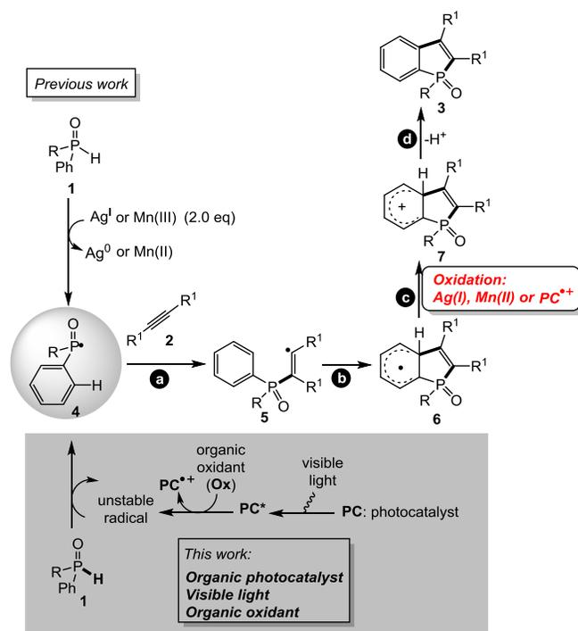
**Scheme 1.** Synthesis of benzo[*b*]phosphole oxides **3** through silver or manganese-mediated processes (previous work) and visible photoredox approach (this work).
