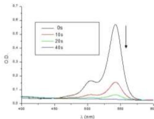
**Figure 4.** Changes in the UV-visible absorption spectrum of a DMF solution of **EY-8b** ( $5.9 \times 10^{-6}$  M) under light irradiation ( $\lambda_{\text{max}} = 530 \text{ nm}$ )-aerated solution.
