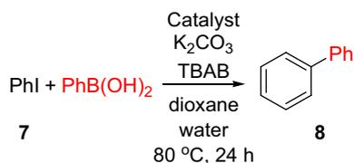
**Scheme 3** Synthesis of biphenyl by Suzuki–Miyaura reaction with the prepared catalysts
