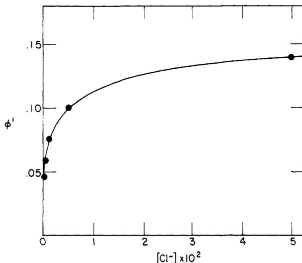
**Figure 5.** The observed initial quantum yield  $\phi'$  for the formation of  $MV^+\cdot Cl^-$  in  $CH_3OH$  vs. the  $Cl^-$  concentration ( $[MV^{2+}(Cl^-)_2] = 4 \times 10^{-5}M$ ; 248.8-nm excitation wavelength).
