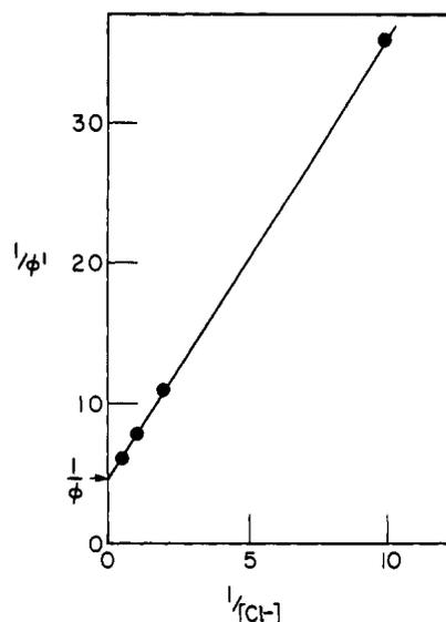
Figure 4. The inverse of the observed quantum yield  $\phi'$  of  $MV^+\cdot Cl_2^-$  formation is plotted vs. the inverse of the  $Cl^-$  concentration present in a 0.1 M phosphate buffer (pH 7) solution ( $[MV^{2+}(Cl^-)_2] = 4 \times 10^{-5}$  M; 248.8-nm excitation wavelength).
