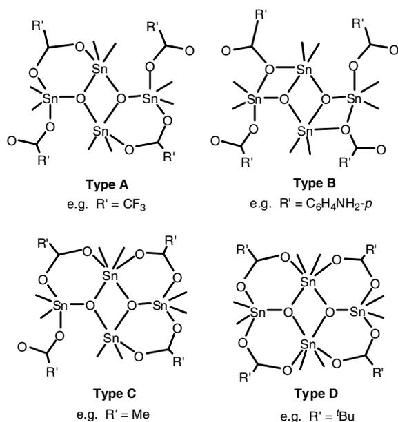
Fig. 1. Four different structural types of  $[(\text{R}_2\text{Sn}(\text{R}'\text{COO})_2)_2\text{O}]_2$ .
