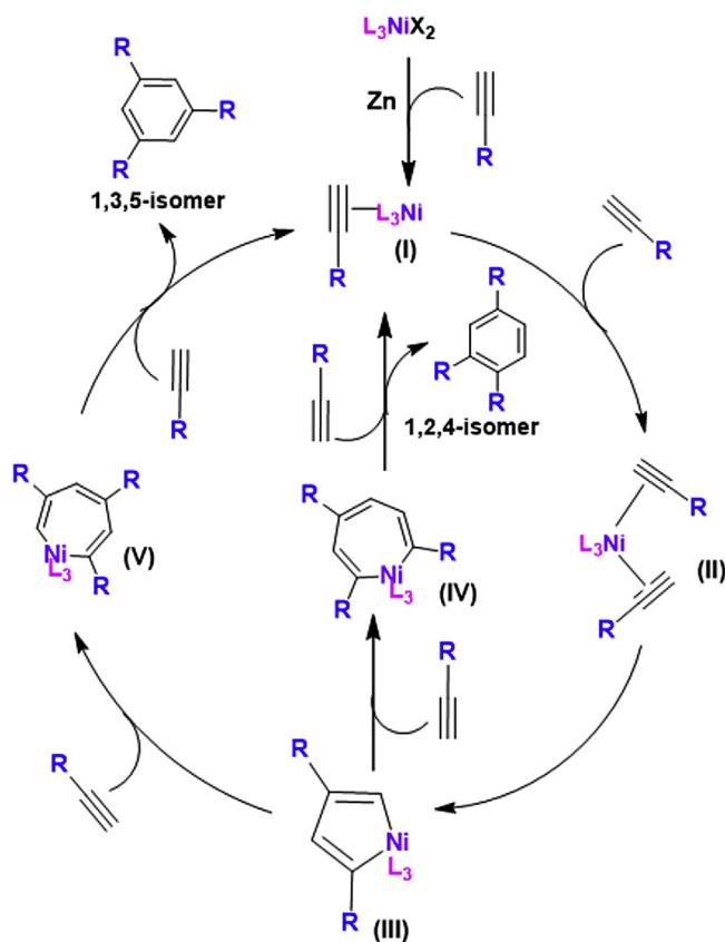
**Scheme 2.** The proposed catalytic cycle for alkynes [2+2+2] cycloaddition.
