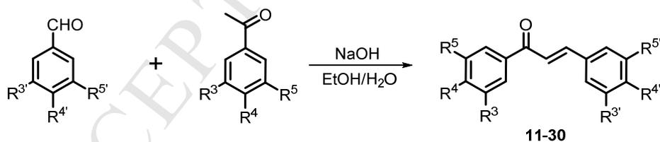
**Scheme 2.** Claisen-Schmidt condensation between substituted benzaldehydes and acetophenones.
