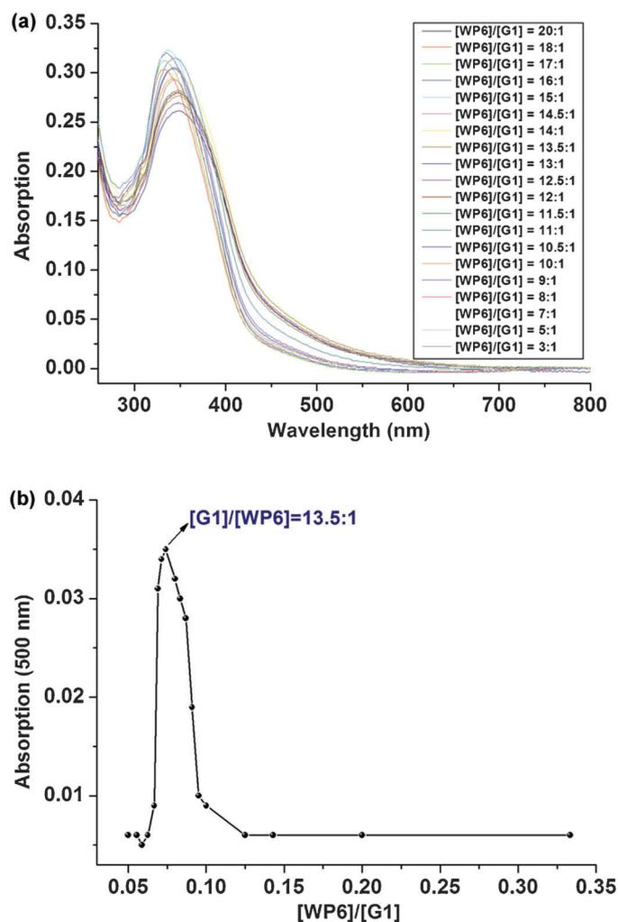
**Figure 3.** a) UV/Vis absorption of a mixture of WP6 and G1 in water with constant G1 concentration (0.02 mM) on increasing the concentration of WP6 (0.05–0.33 equiv) at 25 °C. b) Dependence of the relative absorption intensity at 500 nm on the WP6 concentration with a fixed concentration of G1 (0.02 mM) at 25 °C.
