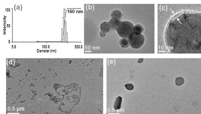
**Figure 4.** a) DLS data of the WP6>G2 aggregates. b)–e) TEM images: b) WP6>G2 aggregates; c) enlarged image of b); d) WP6>G2 aggregates after the solution pH was adjusted to 6.2; e) WP6>G2 aggregates after the solution pH was adjusted back to 7.4. [WP6] =  $1.11 \times 10^{-5}$  M and [G2] =  $1.0 \times 10^{-4}$  M.
