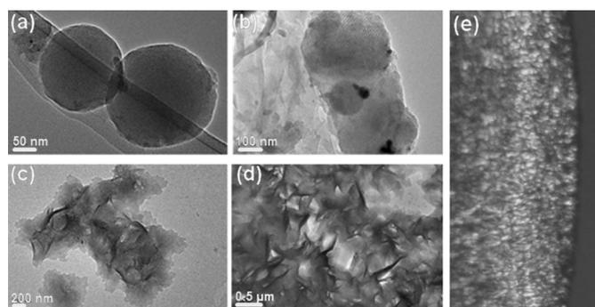
**Figure 2.** TEM images of spherical micelles formed from **WP6** and **G1** gradually converted to layered structures: the samples prepared after a) 0, b) 3, c) 7, and d) 14 days. e) Representative POM image under crossed polarizers of d). [**WP6**] =  $4.35 \times 10^{-6} \text{ M}$  and [**G1**] =  $5.0 \times 10^{-5} \text{ M}$ . Scale bars: a) 50 nm, b) 100 nm, c) 200 nm, d) 0.5 μm.
