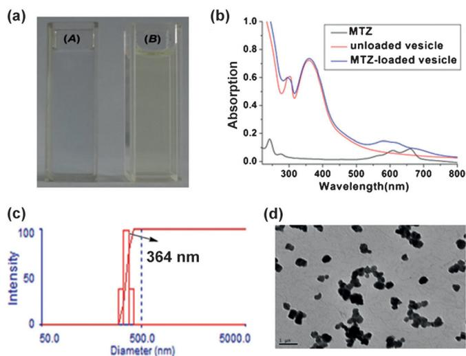
**Figure 6.** a) Color change of MTZ-loaded vesicles (A) compared with unloaded vesicles (B). b) UV/Vis absorption spectra of the solution of MTZ, unloaded vesicles, and MTZ-loaded vesicles at 25 °C in water. c) DLS data of MTZ-loaded vesicles. d) TEM image of MTZ-loaded vesicles.
