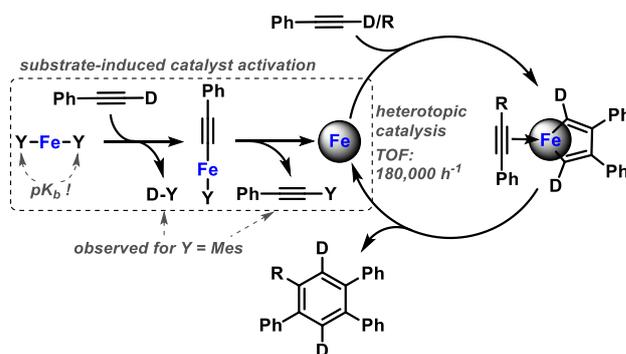
**Scheme 5.** Postulated mechanism involving dual catalyst activation and heterotopic cyclotrimerization catalysis.
