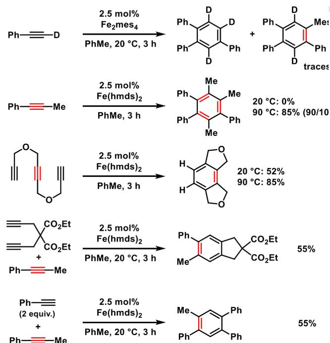
**Scheme 3.** Fe(hmnds)<sub>2</sub>-catalyzed co-cyclizations with internal alkynes.
