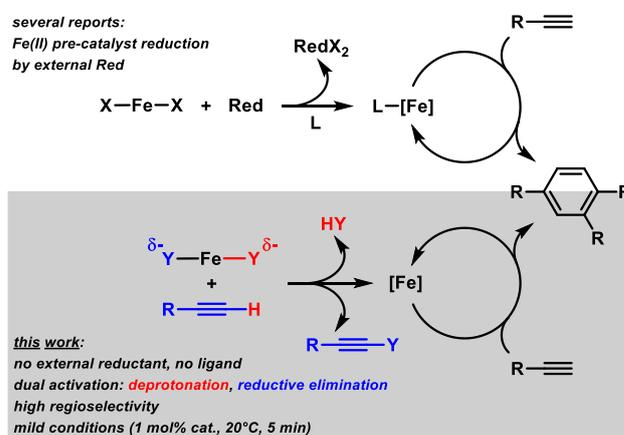
**Scheme 1.** Modes of catalyst formation in iron-catalyzed cyclotrimerization
