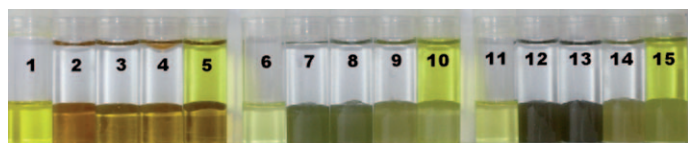
Figure 3. Visual color changes induced by the addition of 2 mL of 0.1 mM solutions of 4 , 5 , and 6 in CHCl 3 to 3 mL of 0.2 mM aqueous solutions of the test nitroaromatic explosives TNB, TNP, and TNT in the absence and presence of salts. Here, “salts” refers to a mixture of NaHCO 3 , K 2 CO 3 , MgSO 4 , CaCl 2 , and NH 4 Cl, 2 mM in each experiment. The contents of the vials from left to right are as follows: 1) pure 4 , 2) 4 + TNB, 3) 4 + TNB + salts, 4) 4 + TNT, 5) 4 + TNP, 6) pure 5 , 7) 5 + TNB, 8) 5 + TNB + salts, 9) 5 + TNT, 10) 5 + TNP, 11) pure 6 , 12) 6 + TNB, 13) 6 + TNB + salts, 14) 6 + TNT, 15) 6 + TNP.
