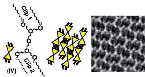
**Figure 3.** Polymerlike topology imposed by a different elongated rigid core. Molecular structure of IV (left), anticipated self-assembly scheme (middle), and obtained STM image (right) corresponding to bifunctional molecules based on an elongated core. The average tunnel current was  $I_T \approx 12$  pA and the sample bias was  $V_T \approx -1.0$  V. The scanned area was  $8.0 \times 8.0$  nm<sup>2</sup>.
