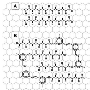
**Figure 1.** Clip design and principle. A) Linear *n*-alkane adsorption in correspondence with HOPG after the Groszek model,<sup>[24]</sup> and B) clip adsorption showing the rigorous preservation of the Groszek structure for the *n*-alkyl chains.
