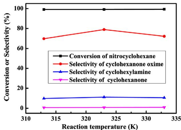
Fig. 4. Effect of reaction temperature on nitrocyclohexane hydrogenation.
