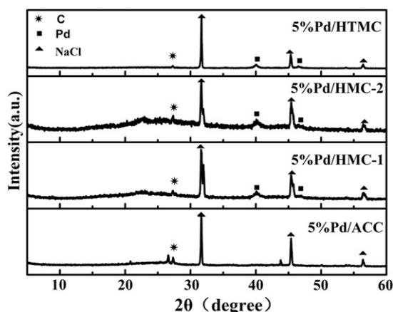
Fig. 3. XRD patterns of 5% Pd/ACC, 5% Pd/HMC-1, 5% Pd/HMC-2 and 5% Pd/HTMC.
