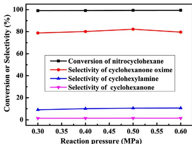
Fig. 5. Effect of reaction pressure on nitrocyclohexane hydrogenation.
