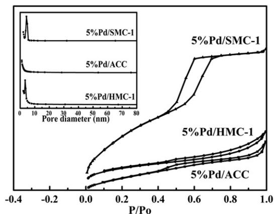
Fig. 1. N<sub>2</sub> adsorption–desorption isotherms and BJH pore size distribution (inset) of 5% Pd/HMC-1, 5% Pd/SMC-1 and 5% Pd/ACC.
