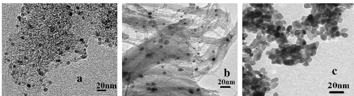
Fig. 2. TEM images of 5% Pd/ACC (a), 5% Pd/HMC-1 (b) and 5% Pd/HTMC (c).
