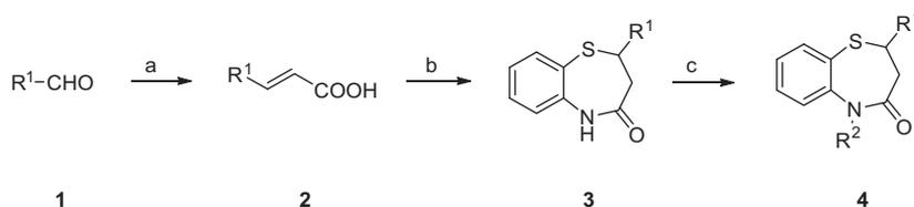
**Scheme 1.** Reagents and conditions: (a)  $\text{CH}_2(\text{COOH})_2$ , pyridine, piperidine, 2 h, reflux, 69–91%; (b) 2-aminobenzenethiol, 4 Å molecular sieve, 6 h, 180 °C, 25–66%; (c)  $\text{R}^2\text{X}$ , X = Cl, Br, I, NaH, DMF, 0.5 h, –10 °C, 11–86%.
