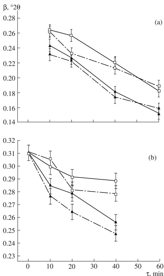
**Fig. 2.** Physical broadening of (a) (104)  $\alpha\text{-Fe}_2\text{O}_3$  and (b) (220)  $\text{NiFe}_2\text{O}_4$  diffraction peaks vs. time of microwave heating (solid lines) and thermal heating (dashed-and-dotted lines):  $\blacktriangle$  850 and  $\square$  900°C.
