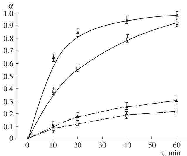
**Fig. 1.** Rate curves for reaction (1) under microwave heating (solid lines) and thermal heating (dashed-and-dotted lines):  $\blacktriangle$  850 and  $\square$  900°C.
