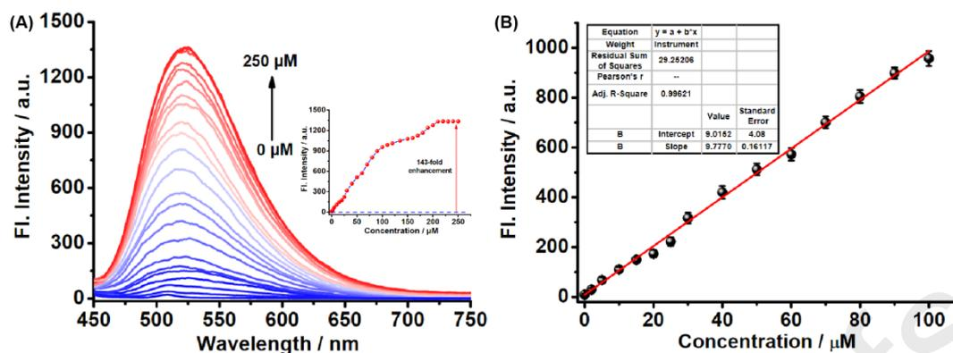
**Fig. 1.** (A) Fluorescent curves of **Na-CM-ER** (10  $\mu\text{M}$ ) encountering with CORM-2 (0-250  $\mu\text{M}$ ) in 10 mM PBS buffer (pH 7.4, 10 % DMSO v/v). Inset shows the fluorescent intensity changes of **Na-CM-ER** (10  $\mu\text{M}$ ) at  $I_{520}$  with CORM-2 (0-250  $\mu\text{M}$ ). (B) Linear relationship of between intensity and CORM-2 concentration.  $\lambda_{\text{ex}} = 430$  nm. Error bars represent standard deviation ( $\pm$ S.D.),  $n = 3$ .
