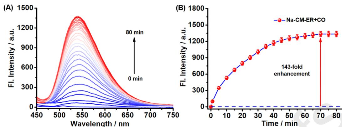
**Fig. 2.** (A) Time-dependent fluorescence spectra of **Na-CM-ER** ( $10 \mu\text{M}$ ) treated with **CORM-2** ( $210 \mu\text{M}$ ). (B) Fluorescent intensity changes of **Na-CM-ER** at  $I_{520}$  treated with **CORM-2** ( $210 \mu\text{M}$ ). Error bars represent standard deviation ( $\pm\text{S.D.}$ ),  $n=3$ .  $\lambda_{\text{ex}} = 430 \text{ nm}$ .
