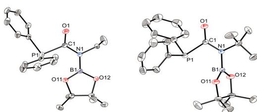
**Fig. 3.** The molecular structures of **6a** and **8a** drawn at the 50% probability level and hydrogen atoms omitted for clarity. Selected bond distances (Å) and angles (°): [6a] C(1)-O(1) 1.2156(14), C(1)-N(1) 1.3820(13), C(1)-P(1) 1.8927(12), N(1)-B(1) 1.4424(14), N(1)-C(20) 1.4822(13); C(1)-N(1)-B(1) 126.03(9), C(1)-N(1)-C(20) 116.25(9), B(1)-N(1)-C(20) 117.71(9). [8a] C(1)-O(1) 1.2235(13), C(1)-N(1) 1.3570(14), C(1)-P(1) 1.8894(11), N(1)-
