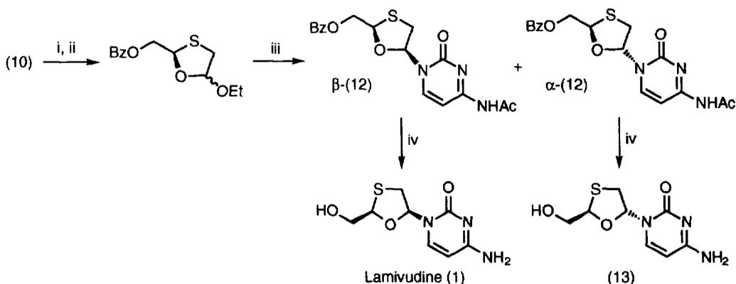
Reagents and conditions: i)  $\text{LiBH}_4$ ,  $^i\text{PrOH}$  (cat.), THF, 96%; ii)  $\text{BzCl}$ , pyridine,  $\text{CH}_2\text{Cl}_2$ , 88%; iii) Silylated N-acetyl cytosine (11), TMSOTf,  $\text{CH}_3\text{CN}$ , 43%; iv)  $\text{NH}_3$ , MeOH, 98% (both anomers).
