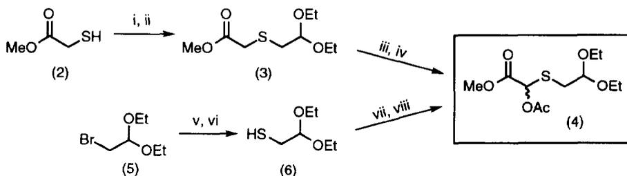
Reagents and conditions: i) Na, DMF; ii)  $\text{BrCH}_2\text{CH}(\text{OEt})_2$ , 52%; iii) *m*-CPBA,  $\text{CH}_2\text{Cl}_2$ , 96%; iv)  $\text{Ac}_2\text{O}$ , NaOAc, 90 °C, 81%; v)  $\text{KSC}(\text{S})\text{OEt}$ , acetone, 95%; vi)  $\text{H}_2\text{NCH}_2\text{CH}_2\text{NH}_2$ , 91%; vii)  $\text{MeOC}(\text{O})\text{CHO}$ ,  $\text{CH}_2\text{Cl}_2$ , 4Å sieves; viii)  $\text{Ac}_2\text{O}$ , pyridine, DMAP, 73%.
