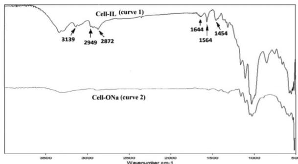
Fig. 1 FT-IR spectra comparison of Cell-ONa and immobilized IL.
