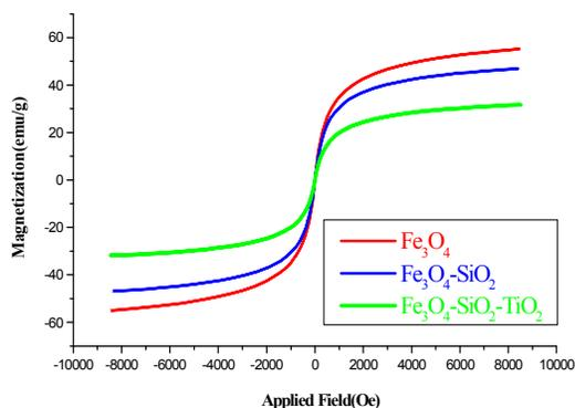
**Figure 5.** Magnetization curves for the  $\text{Fe}_3\text{O}_4$  (red line),  $\text{Fe}_3\text{O}_4@ \text{SiO}_2$  (blue line) and  $\text{Fe}_3\text{O}_4@ \text{SiO}_2\text{-TiO}_2$  (green line) at room temperature.
