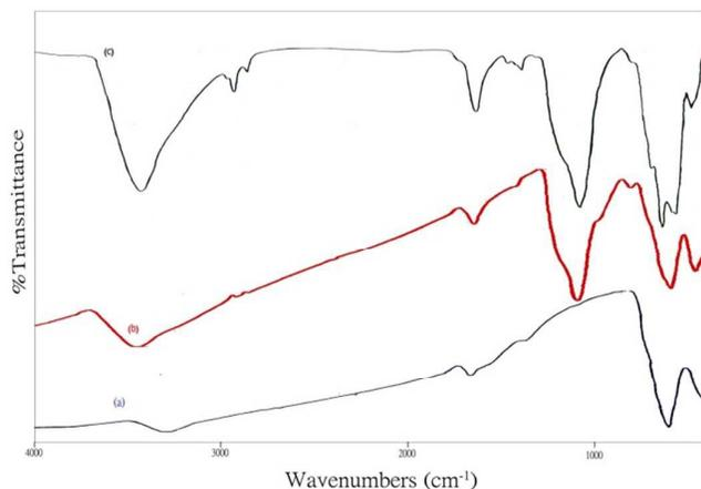
**Figure 4.** FT-IR spectra of (a)  $\text{Fe}_3\text{O}_4$ , (b)  $\text{Fe}_3\text{O}_4@ \text{SiO}_2$  and (c)  $\text{Fe}_3\text{O}_4@ \text{SiO}_2\text{-TiO}_2$ .
