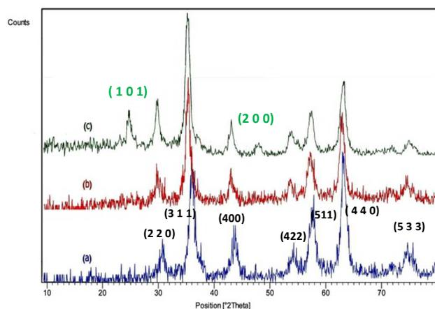
**Figure 1.** The XRD patterns of (a)  $\text{Fe}_3\text{O}_4$  (b)  $\text{Fe}_3\text{O}_4@SiO_2$  and (c)  $\text{Fe}_3\text{O}_4@SiO_2-TiO_2$ .
