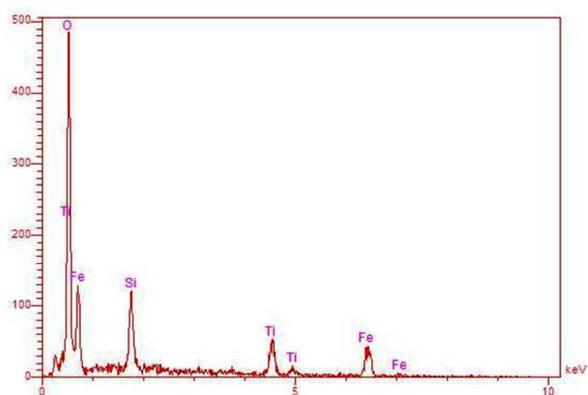
**Figure 2.** The EDAX of  $\text{Fe}_3\text{O}_4@SiO_2-TiO_2$  nanocatalyst.
