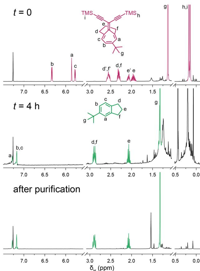
**Figure 2.** <sup>1</sup>H NMR spectra (CDCl<sub>3</sub>, 298 K, 400 MHz) of UV unmasking (250 nm) of **12** in CDCl<sub>3</sub>.
