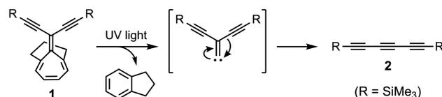
**Scheme 1.** Photochemical unmasking of bicyclo[4.3.1]deca-1,5-diene **1** and subsequent rearrangement of the carbene to form TMS-triynes **2**.<sup>[15]</sup>
