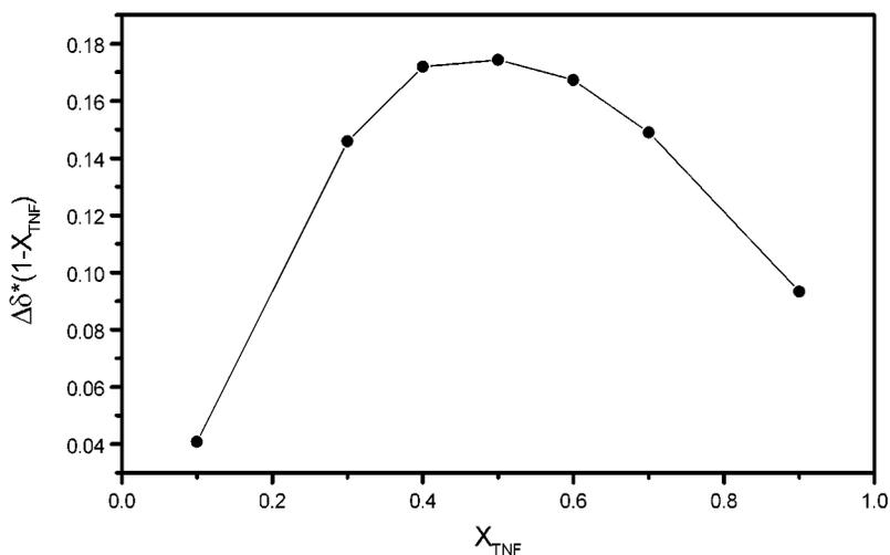
**Figure 2.** Job plot of the chemical shift change of the *N*-methyl groups of the tweezer molecule (**4**) as a function of the mole fraction of 2,4,7-trinitrofluorenone in  $\text{CDCl}_3$  showing the 1:1 binding stoichiometry.
