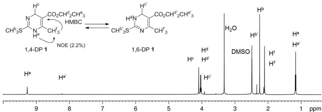
Fig. 4.  $^1\text{H}$  NMR spectrum of dihydropyrimidine 1 [DMSO- $d_6$ , 0.012 M, 20 °C (293 K)].
