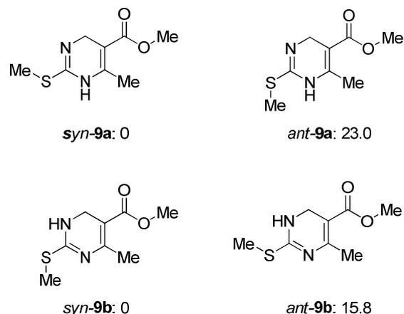
Fig. 12. Two energy-minimum conformers of **9a** and **9b**. Values are relative energies to the *syn* forms in kJ mol<sup>-1</sup>.
