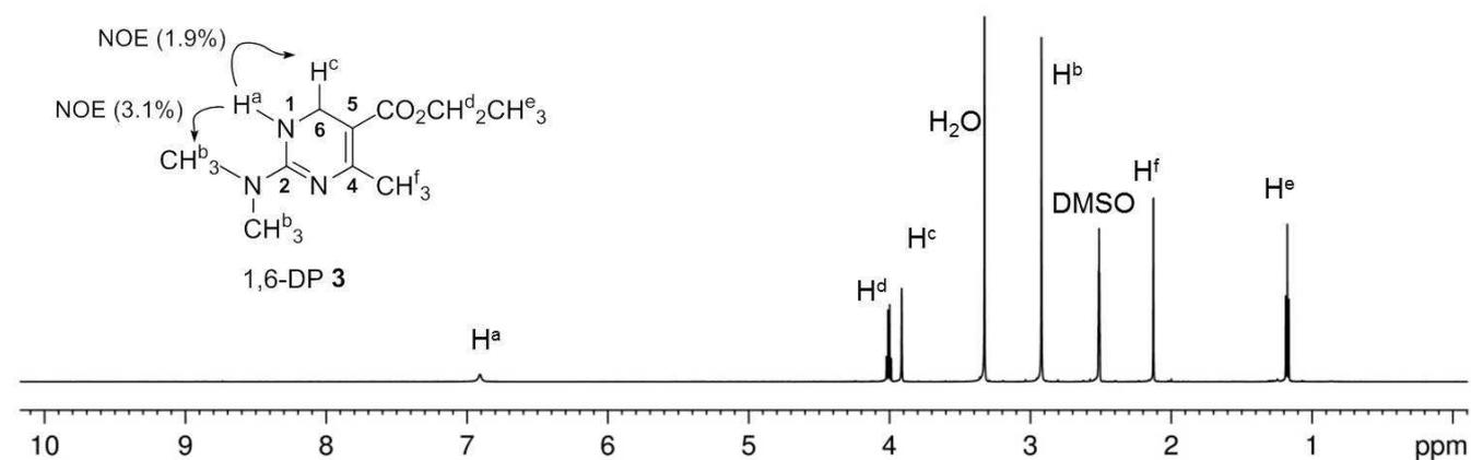
Fig. 6.  $^1\text{H}$  NMR spectrum of dihydropyrimidine 3 [DMSO- $d_6$ , 0.012 M, 25 °C (298 K)].
