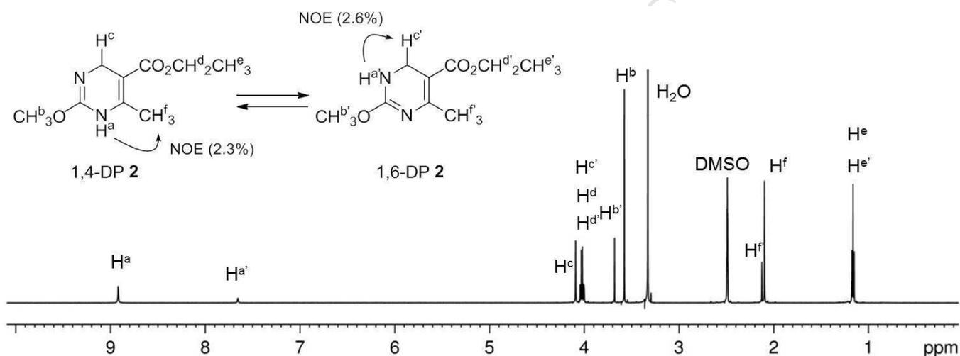
Fig. 5.  $^1\text{H}$  NMR spectrum of dihydropyrimidine 2 [DMSO- $d_6$ , 0.012 M, 20 °C (293 K)].
