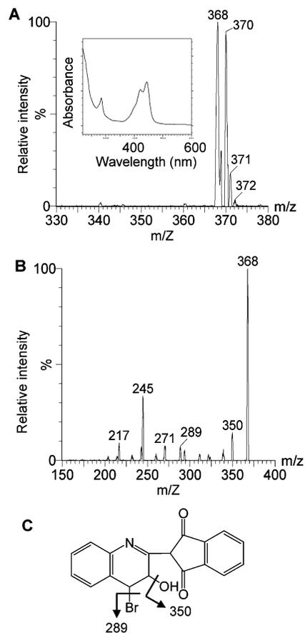
**FIGURE 5.** (A) MS spectrum and the UV spectrum in methanol ( $\lambda_{\max}$ : 443, 422, 285 nm) of Y2. (B) MS/MS spectrum of the  $[M + H]^+$  ion 368 of Y2. (C) Chemical structure of DY 64.
