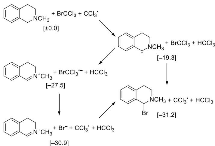
**Scheme 10.** Radical chain reaction via trichloromethyl radicals with *N*-methyl tetrahydroisoquinoline as substrate, relative free energies in kcal/mol (same level of theory as in Scheme 7).
