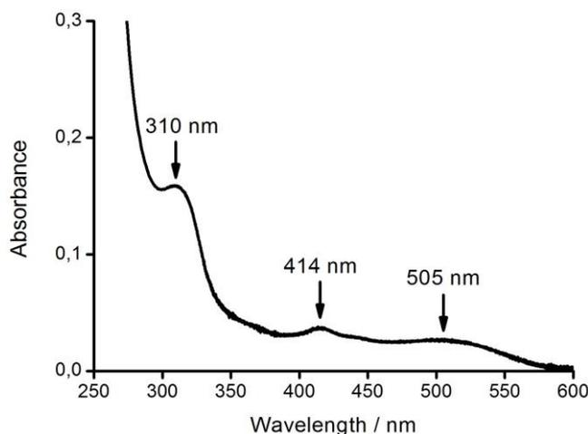
**Figure 1.** UV/vis spectrum of the reaction mixture of **8** and  $\text{BrCCl}_3$  showing absorption maxima of polymethinecyanines.
