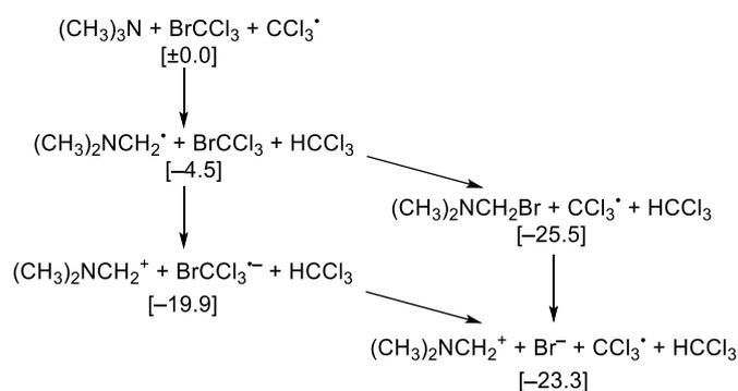
**Scheme 9.** Radical chain reaction via trichloromethyl radicals with trimethylamine as substrate, relative free energies in kcal/mol (same level of theory as in Scheme 6, the “ $(\text{CH}_3)_2\text{NCH}_2\text{Br}$ ” should be regarded as a contact ion pair).
