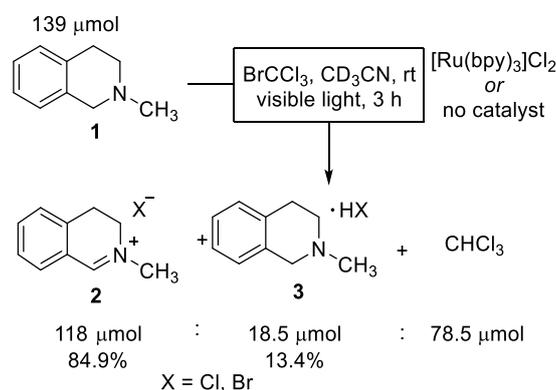
**Scheme 1.** Photogeneration of iminium ions. Amounts were quantified by  $^1\text{H}$  NMR spectroscopy with an internal standard.
