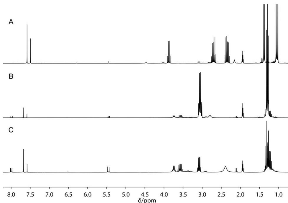
**Figure 2.** Crude <sup>1</sup>H NMR spectra (acetonitrile-*d*<sub>3</sub>) of the triethylamine oxidation with different additives: (A) Potassium cyanide as an additive results in  $\alpha$ -aminonitrile formation. (B) Without additive, the amine hydrohalide and the cyanine dye are formed. (C) Addition of potassium carbonate results in the accumulation of the cyanine dye.
