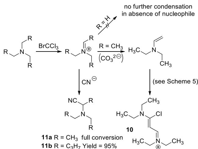
**Scheme 6.** Reaction pathway of oxidized aliphatic amines with additives
