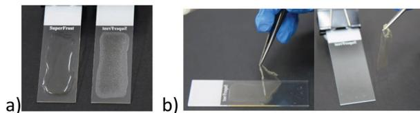
Fig. 6 (a) A gel, directly after application (left) and after 24 hours (right). (b) Peeling the film from a glass surface.
