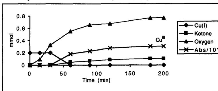
Cyclohexane 10 mmol, Cu(CH<sub>3</sub>CN)ClO<sub>4</sub> 0.2 mmol, H<sub>2</sub>O<sub>2</sub> 2 mmol, Pyridine 33 ml, 0°C to room temperature.
