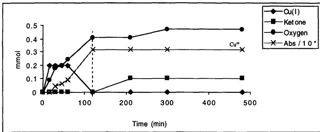
Cyclohexane 10 mmol,  $\text{Cu}(\text{ClO}_4)_2 \cdot 6\text{H}_2\text{O}$  0.2 mmol,  $\text{H}_2\text{O}_2$  2 mmol, Pyridine 33 ml,  $0^\circ\text{C}$  to room temperature.
