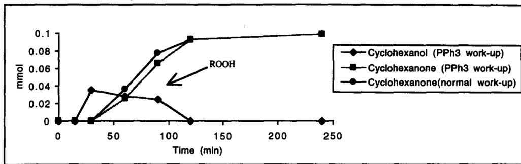
Cyclohexane 10 mmol,  $\text{Cu}(\text{ClO}_4)_2 \cdot 6\text{H}_2\text{O}$  0.2 mmol,  $\text{H}_2\text{O}_2$  2 mmol, Pyridine 33 ml, from  $0^\circ\text{C}$  to room temperature.
