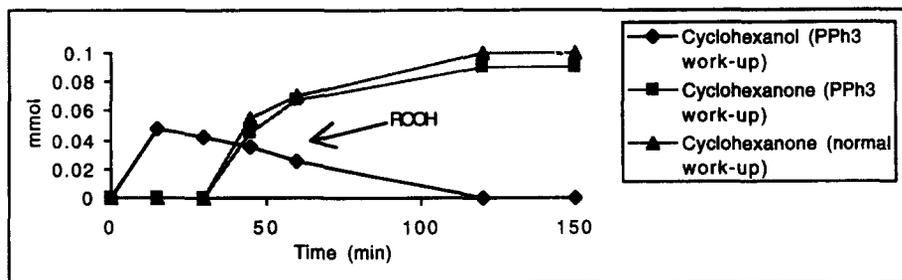
Cyclohexane 10 mmol, solution of Cu<sup>III</sup> species (λ<sub>max</sub>= 472 nm) 0.2 mmol, H<sub>2</sub>O<sub>2</sub> 2 mmol, Pyridine 33 ml, from 0°C to room temperature.
