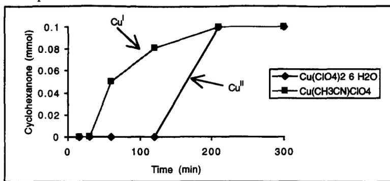
Cyclohexane 10 mmol, copper salt 0.2 mmol, H<sub>2</sub>O<sub>2</sub> 2 mmol, Pyridine 33 ml, under argon from 0°C to room temperature
