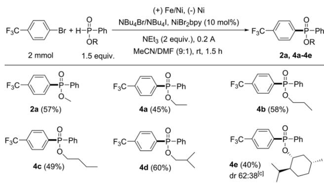
[a] Typical procedure: undivided cell, iron/nickel (64/36) anode, nickel cathode, tetrabutylammonium bromide/tetrabutylammonium iodide (0.15 mmol/0.068 mmol), acetonitrile/DMF (18/2 mL, v/v), NiBr<sub>2</sub>.bpy (10 mol-%), 4-bromobenzotrifluoride (2 mmol), alkyl *H*-phenylphosphinate (3 mmol), triethylamine (4 mmol), constant current: 200 mA, room temperature. [b] Isolated yield. [c] Diastereomeric ratio (dr) was determined by <sup>1</sup>H NMR.
