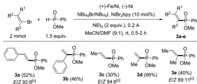
[a] Typical procedure: undivided cell, iron/nickel (64/36) anode, nickel cathode, tetrabutylammonium bromide/tetrabutylammonium iodide (0.15 mmol/0.068 mmol), acetonitrile/DMF (18/2 mL, v/v), NiBr<sub>2</sub>.bpy (10 mol-%), vinyl bromide (2 mmol), methyl *H*-phenylphosphinate (3 mmol), triethylamine (4 mmol), constant current: 200 mA, room temperature. [b] Isolated yield. [c] E/Z ratio was determined by <sup>31</sup>P NMR.
