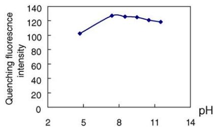
Fig. 4. The pH effect of the final determination ( $C_{\text{TMAPABODIPY}} = 6.0 \times 10^{-5} \text{ mol l}^{-1}$ ,  $C_{\text{NO}} = 2.00 \times 10^{-6} \text{ mol l}^{-1}$ , reaction time: 30 min, reaction temperature:  $30^\circ\text{C}$ ).
