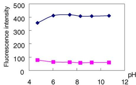
Fig. 2. Effect of pH on the fluorescence intensity of TMAPABODIPY and TMAPABODIPY-T.  $C_{\text{TMAPABODIPY}} = 6.0 \times 10^{-6} \text{ mol l}^{-1}$ ,  $C_{\text{NO}} = 2.00 \times 10^{-5} \text{ mol l}^{-1}$ , (◆) TMAPABODIPY, (■) TMAPABODIPY-T.
