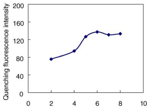
Fig. 3. Effect of TMAPABODIPY concentration ( $C_{\text{NO}} = 2.00 \times 10^{-6} \text{ mol l}^{-1}$ , pH 7.40, reaction time: 30 min, reaction temperature:  $30^\circ\text{C}$ ).
