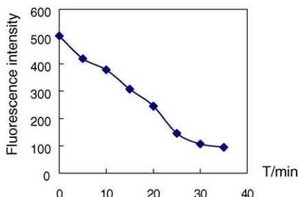
Fig. 7. The time course of the decrease of the fluorescence intensity at 510 nm of the fluorescence probe ( $C_{\text{TMAPABODIPY}} = 6.0 \times 10^{-5} \text{ mol l}^{-1}$ ). A spontaneous NO-releasing reagent, *S*-nitrosocysteine was added to probe solution at a final concentration of  $7.5 \mu\text{mol l}^{-1}$  at 0 min.
