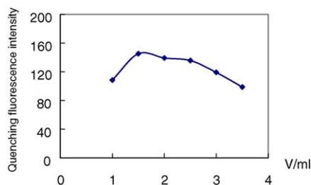
Fig. 5. Effect of buffer volume ( $C_{\text{TMAPABODIPY}} = 6.0 \times 10^{-5} \text{ mol l}^{-1}$ ,  $C_{\text{NO}} = 2.00 \times 10^{-6} \text{ mol l}^{-1}$ , pH 7.40, reaction time: 30 min, reaction temperature:  $30^\circ\text{C}$ ).
