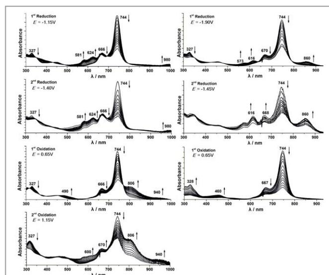
**Figure 7** Thin-layer spectroelectrochemistry of **3a** in *o*-dichlorobenzene (left side) and DMF (right side) containing 0.1M TBAP.
