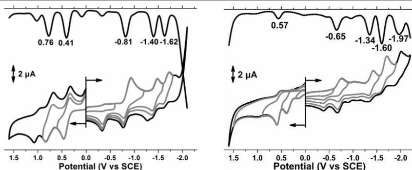
**Figure 4** DPV and CV data for **2** in *o*-dichlorobenzene (left) and DMF (right) containing 0.1 M TBAP, scan rate = 100 mV/s.
