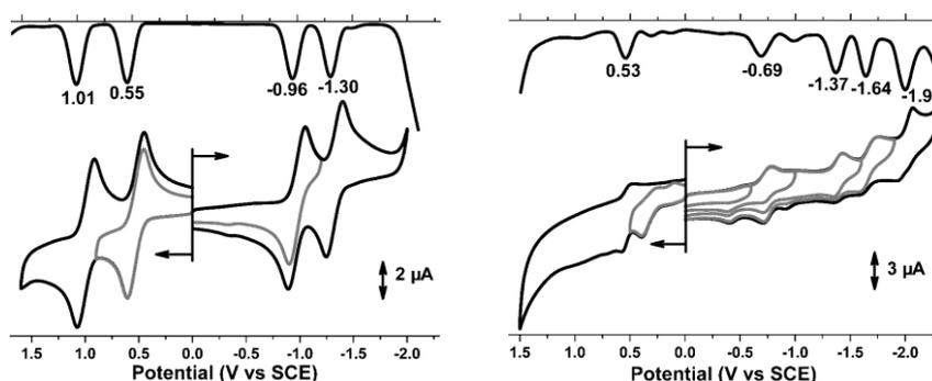
**Figure 5** DPV and CV data for **3a** in *o*-dichlorobenzene (left) and DMF (right) containing 0.1 M TBAP, scan rate = 100 mV/s.
