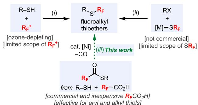
**Figure 1.** (A) Representative examples of bioactive molecules containing fluoroalkyl thioethers ( $R_FSR$ ). (B) Existing synthetic approaches to  $R_FSR$  (i, ii) and our approach (iii).
