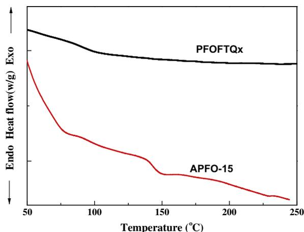
Fig. 2. DSC scans of polymers at a heating rate of 20 °C/min in nitrogen.
