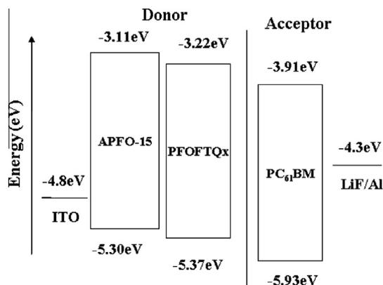
**Fig. 5.** Energy level diagrams of synthesized APFO-15, PFOFTQx and PC<sub>61</sub>BM.
