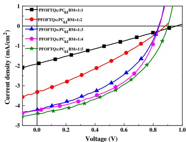
**Fig. 7.**  $J$ - $V$  curves of the PSCs based on PFOFTQx:PC<sub>61</sub>BM with different donor/acceptor weight ratios (1:1, 1:2, 1:3, 1:4 and 1:5), under illumination of AM1.5G, 100 mW/cm<sup>2</sup>.
