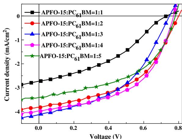
**Fig. 6.**  $J$ - $V$  curves of the PSCs based on synthesized APFO-15:PC<sub>61</sub>BM with different donor/acceptor weight ratios (1:1, 1:2, 1:3, 1:4 and 1:5), under illumination of AM1.5G, 100 mW/cm<sup>2</sup>.
