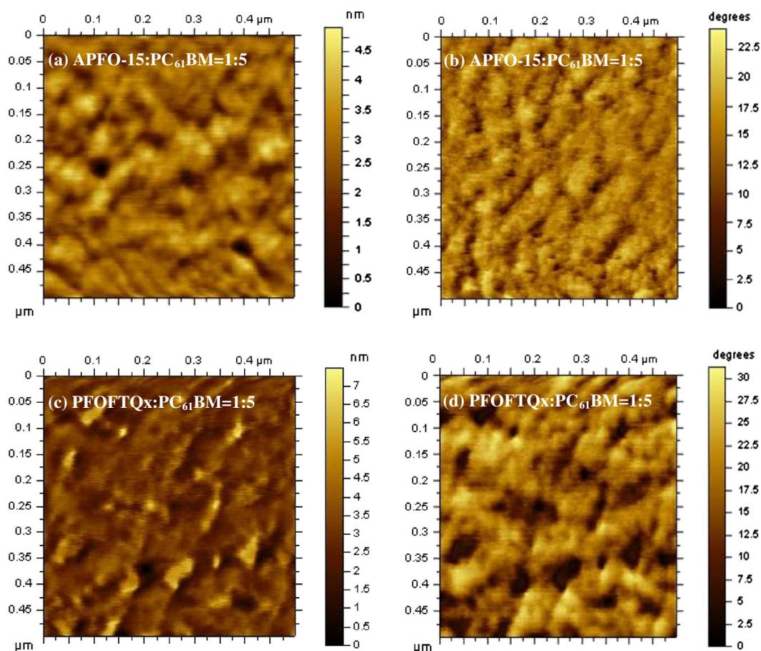
**Fig. 8.** AFM images for polymer:PC<sub>61</sub>BM films (1:5) (0.5 μm × 0.5 μm). (a and c) The topography of polymer film. (b and d) The corresponding phase images.
