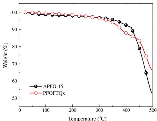
Fig. 1. Thermal gravimetric analysis curves of polymers with a heating rate of 10 °C/min in nitrogen.
