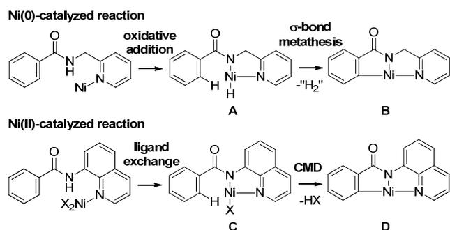
**Scheme 1** Key steps for the activation of C-H bonds by nickel complexes in a bidentate-chelation system. For simplicity, groups that are not involved in the transformation, such as ligands and reagents, are omitted.
