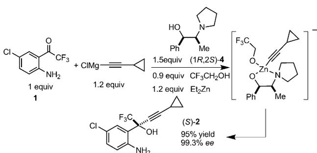
**Scheme 1.** Current “stoichiometric” synthesis of (*S*)-**2**, a key intermediate in the synthesis of efavirenz.
