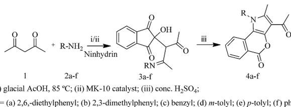
**Scheme 1** Synthesis of 3-acetyl-2-methyl-1-phenylisochromeno [4,3-*b*] pyrrol-5(1*H*)-ones **4a–f**.
