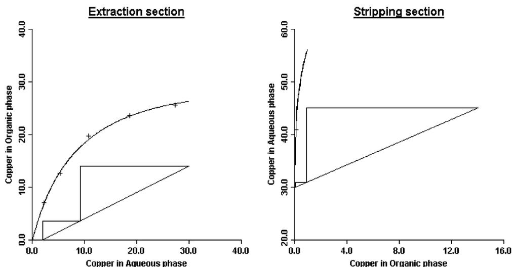
Fig. 5 McCabe–Thiele constructions for the recovery of copper with **7** (1.0 M in Orfom SX7®). All scales in g l<sup>-1</sup>.
