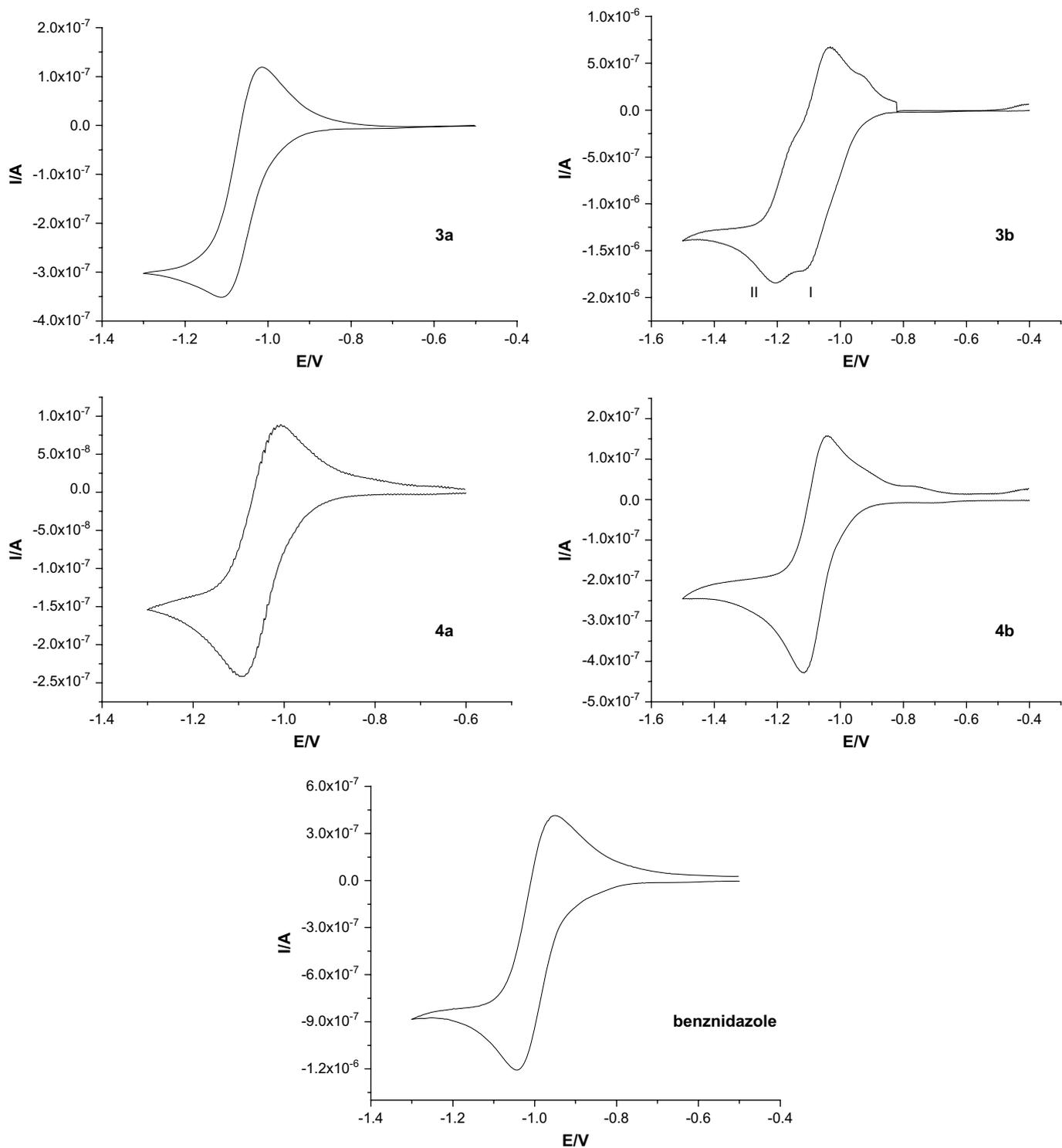
Fig. 3. Cyclic voltammograms at 1 mM in DMF of the compounds **3a,b**, **4a,b** and benznidazole.
