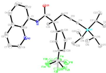
Figure 1. ORTEP of drawing of internal alkyne 3i.
