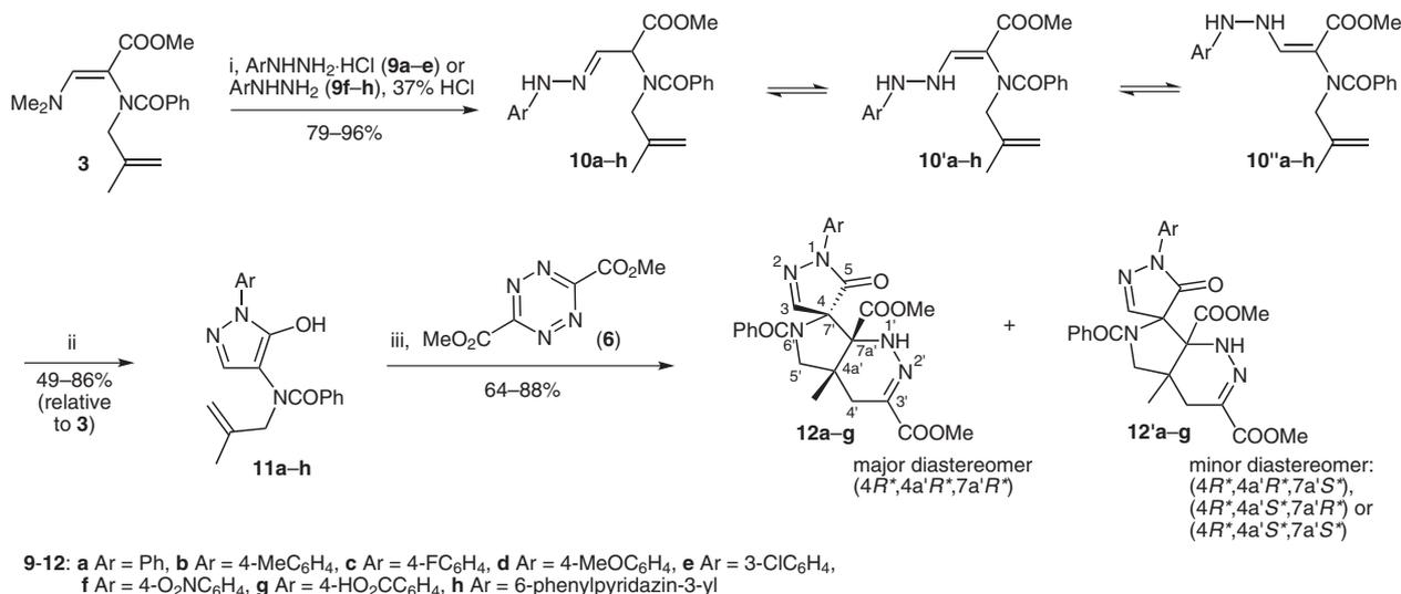
**Scheme 3** Reagents and conditions: (i) EtOH, reflux; (ii) Et<sub>3</sub>N, EtOH, reflux; (iii) MeCN, reflux.
