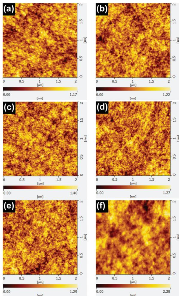
**Fig. 5** Topographic AFM images of (a) PCB-Ph-CB (RMS = 0.184 nm), (b) PCB-C1-CB (RMS = 0.193 nm), (c) PCB-C3-CB, (RMS = 0.212 nm), (d) PCB-C6-CB (RMS = 0.198 nm), (e) PCB-C11-CB (RMS = 0.203 nm), and (f) physical blend of PCBM and 1-(4-*n*-BuC<sub>6</sub>H<sub>4</sub>)-2-Me-1,2-*closo*-C<sub>2</sub>B<sub>10</sub>H<sub>10</sub> (RMS = 0.360 nm).
