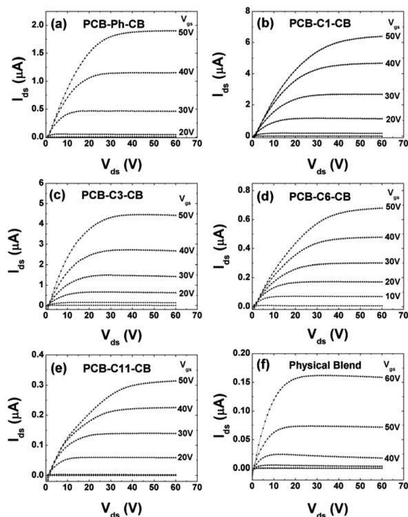
Fig. 4 OFET output characteristics of PCB-Ph-CB and PCB-C<sub>n</sub>-CB.
