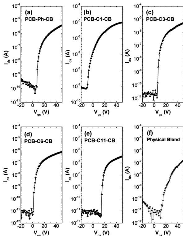
Fig. 3 OFET transfer characteristics of PCB-Ph-CB and PCB-C<sub>n</sub>-CB.
