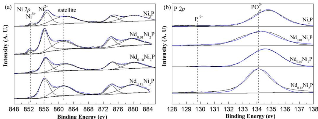
Fig. 2. XPS spectra of the  $\text{Ni}_2\text{P}$  and  $\text{Nd}_x\text{Ni}_2\text{P}$  catalysts.
