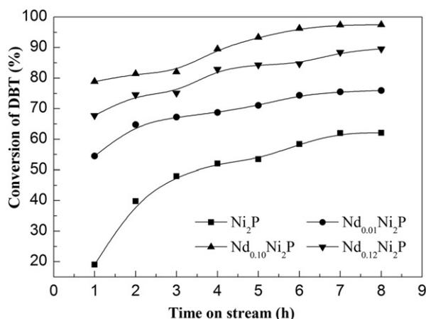
Fig. 3. The HDS activity of the  $\text{Ni}_2\text{P}$  and  $\text{Nd}_x\text{Ni}_2\text{P}$  catalysts. Temperature, 340 °C; pressure, 3.0 MPa;  $\text{H}_2/\text{oil}$  ratio, 500 (V/V); WHSV,  $1.5 \text{ h}^{-1}$ .
