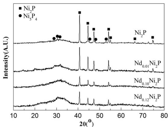
Fig. 1. XRD patterns of the  $\text{Ni}_2\text{P}$  and  $\text{Nd}_x\text{Ni}_2\text{P}$  catalysts.
