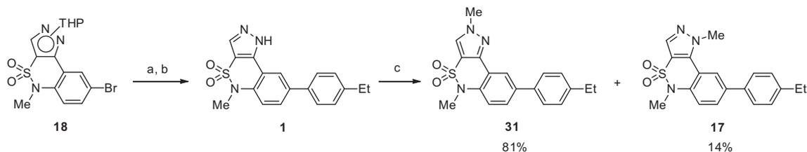
**Scheme 6.** Reagents and conditions: (a) 4-EtPhB(OH)<sub>2</sub>, Pd(OAc)<sub>2</sub>, PPh<sub>3</sub>, Na<sub>2</sub>CO<sub>3</sub>, H<sub>2</sub>O, DME, 150–170 °C, microwave; (b) HCl, MeOH; (c) MeI, K<sub>2</sub>CO<sub>3</sub>, DMF.
