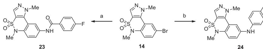
**Scheme 3.** Reagents and conditions: (a) 4-FPhCONH<sub>2</sub>, CuI, *N,N*-dimethylcyclohexane-1,2-diamine, K<sub>2</sub>CO<sub>3</sub>, DMA, 150–180 °C, microwave; (b) 4-FPhNH<sub>2</sub>, Pd<sub>2</sub>(dba)<sub>3</sub>, X-phos, <sup>t</sup>BuONa, DMA, 150 °C, microwave.
