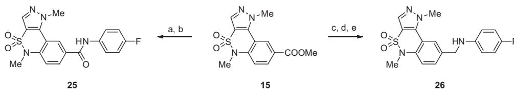
**Scheme 4.** Reagents and conditions: (a) NaOH aq, MeOH; (b) 4-FPhNH<sub>2</sub>, EDC, HOBt, DMF; (c) LiAlH<sub>4</sub>, THF; (d) MsCl, Et<sub>3</sub>N, THF; (e) 4-FPhNH<sub>2</sub>, Et<sub>3</sub>N, THF.
