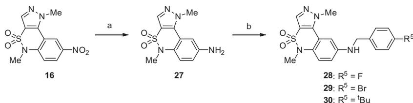
**Scheme 5.** Reagents and conditions: (a) Pd-C, H<sub>2</sub>, MeOH, MeCN; (b) 4-R<sup>5</sup>PhCHO, AcOH, MeCN, DMA, then NaBH<sub>4</sub>.
