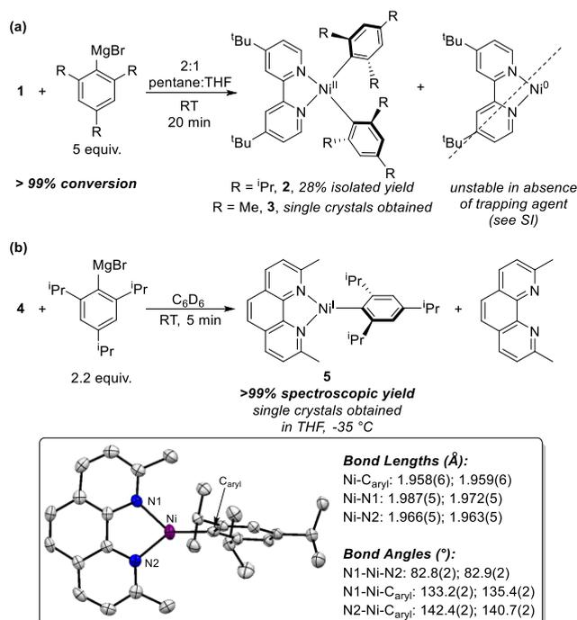
**Scheme 3.** Transmetalation of (a) **1** to produce **2** or **3** and zerovalent Ni; and (b) **4** to produce **5**. Inset: ORTEP of **5**. Ellipsoids shown at 50% probability. Hydrogen atoms and solvent of crystallization omitted. Two independent molecules are present in the asymmetric unit.
