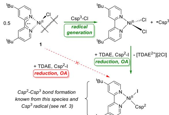
**Scheme 5.** Summary of mechanistic information relevant to cross-electrophile coupling gained from stoichiometric reactions with **1**.
