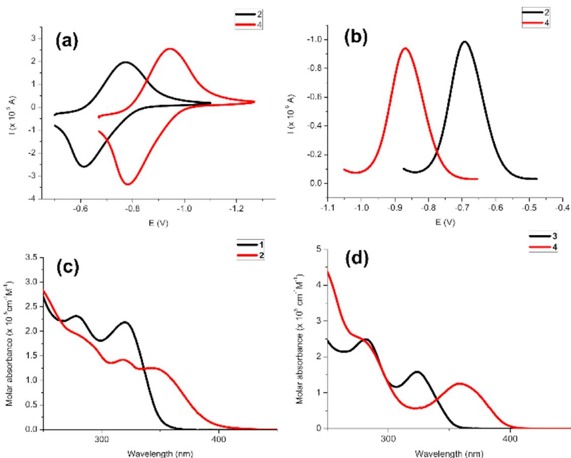
Figure 3. (a) Cyclic voltammograms of **2** and **4** in  $\text{CH}_3\text{CN}$  at 298 K. (b) DPV of **2** and **4** in  $\text{CH}_3\text{CN}$  at 298 K. The concentration of **2** and **4** is  $2.0 \times 10^{-3}$  M. (c) UV/vis spectra of **1** and **2** in  $\text{CH}_3\text{CN}$  at 298 K. (d) UV/vis spectra of **3** and **4** in  $\text{CH}_3\text{CN}$  at 298 K. The concentration of **2** and **4** in (c) and (d) is  $2.0 \times 10^{-5}$  M.
