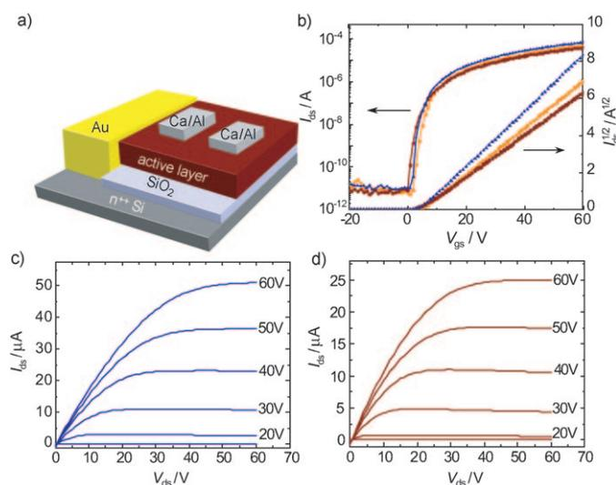
**Figure 2.** a) Schematic diagram of the n-type OFET structure ( $L = 50 \mu\text{m}$ ,  $W = 1.5 \text{ mm}$ ). b) Transfer characteristics in the saturated regime (■; PCBM, ▲; [5,6]-open APCBM, ●; [6,6]-closed APCBM). Output curves at different gate voltages for c) [5,6]-open APCBM and d) [6,6]-closed APCBM.
